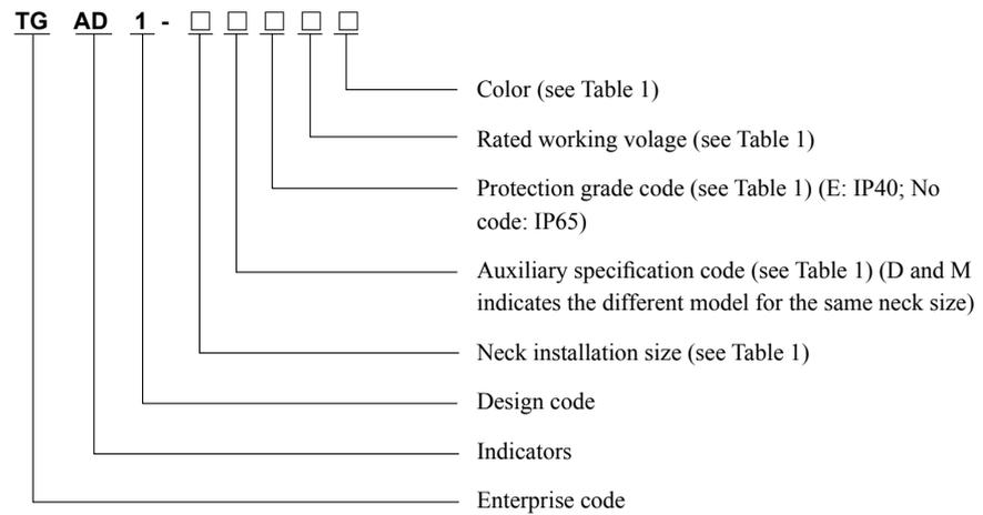
Note: Explanation of auxiliary specification codes (D, M): D indicates an arc round lampshade, and M indicates a buzzer (see Table 1).
